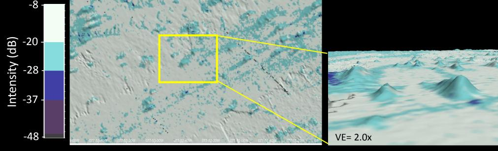
Figure 4c. 2D and 3D classified SIPS backscatter intensity surface draped on bathymetric surface. Note the difference in intensity of backscatter returns from the mounds compared to the surrounding strata.
