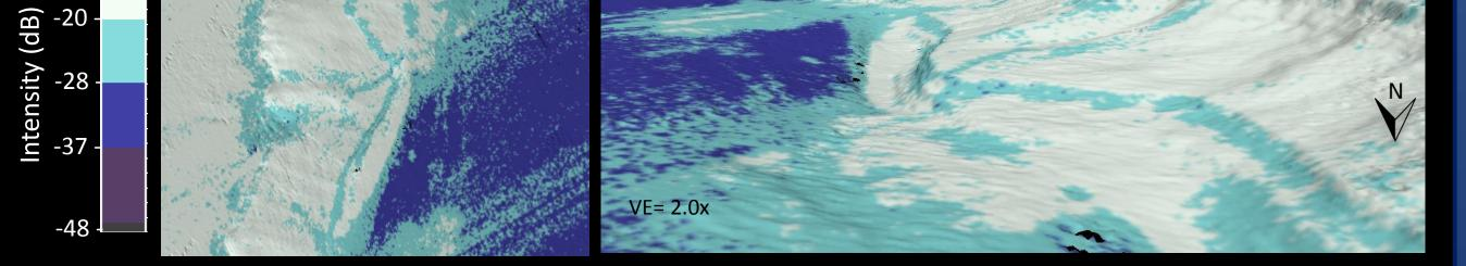
Figure 5c. 2D and 3D classified SIPS backscatter intensity surface draped on bathymetric surface. Note the intensity of backscatter returns on the scarp face compared to that of the flat lying strata below the scarp.
