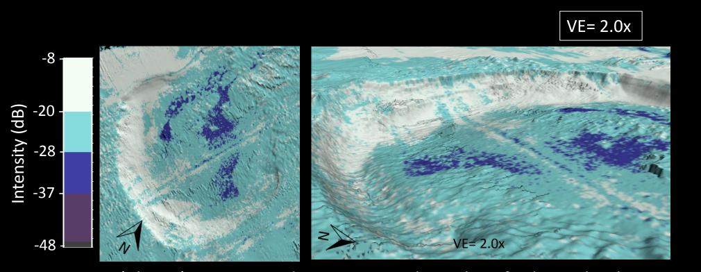
Figure 3c (above). BASIN study area 2D and 3D classified SIPS backscatter intensity surface draped on bathymetric surface. Note the difference in intensity of backscatter returns of the scarp face compared to the basin floor.
