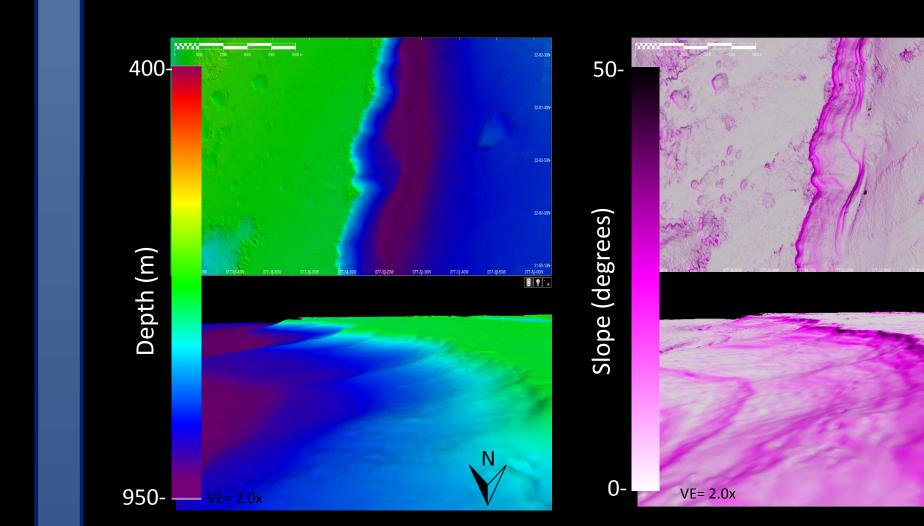
Figure 5b. SCARP Study Area CUBE bathymetric surface with a resolution of 15m. 2D and 3D surface of depth (left) and slope (right). Note the difference in slope of the top of the scarp face compared to the bottom of the scarp face.
